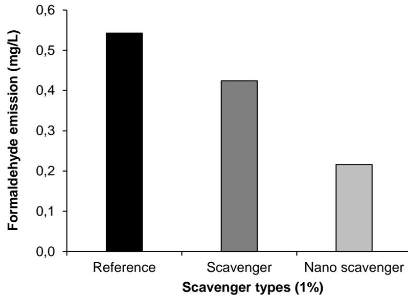
Figure 2. Formaldehyde emission from MDF board having different types of bio-scavenger
