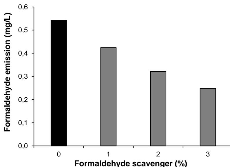
Figure 1. Formaldehyde emission from MDF board having different amount of bio-scavenger
