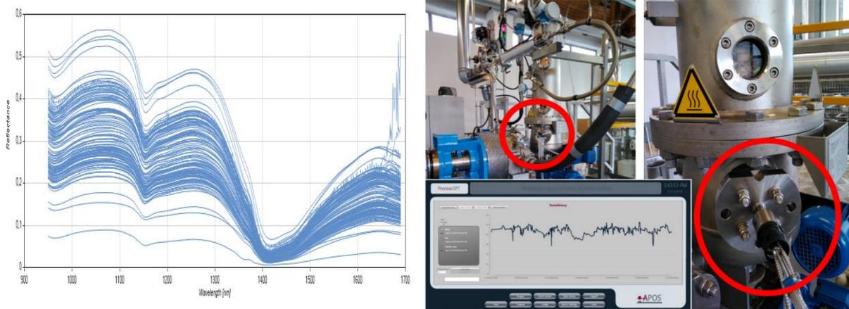
Figure 1: left: NIR spectra, right: ANDRITZ laboratory pilot plant with built-in sensor. Presentation of the measured value (online)
